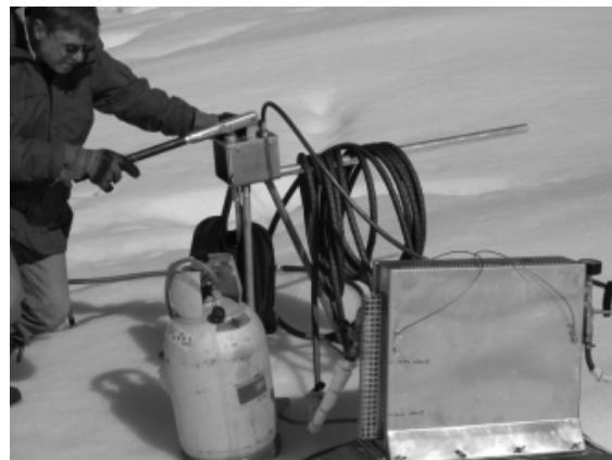
Figure 3. The steam drill in operation in the field.
